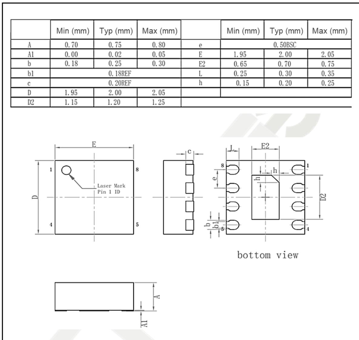
**Figure 17 SOP8 Mechanical Data and Package Dimensions**
