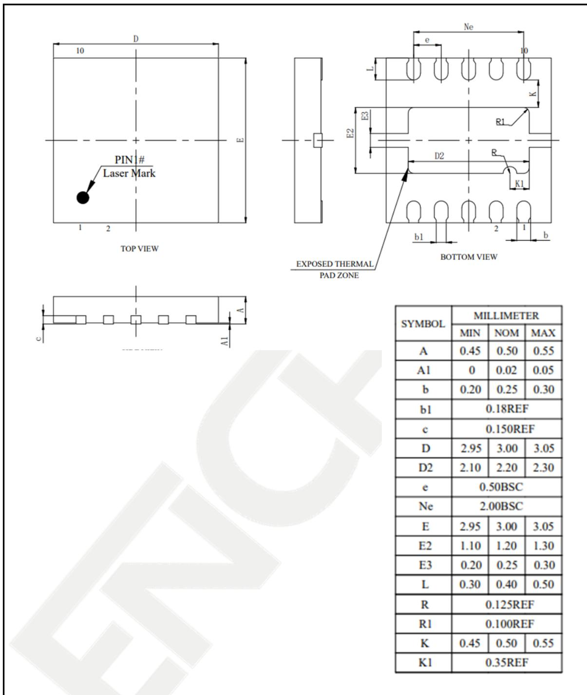
Figure 21 SSOP10 Mechanical Data and Package Dimensions
