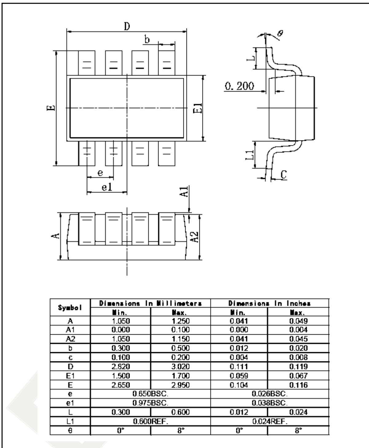
Figure 19 MSOP8 Mechanical Data and Package Dimensions
