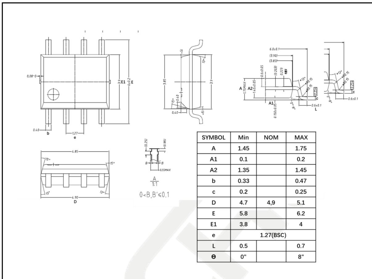
Figure 18 SOT23-8L Mechanical Data and Package Dimensions
